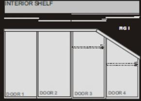
In the above 4 door run, DOOR1 will only move around 65% of its width (up to the angle). DOORS 2 & 3 will move to the left and expose all the space behind. When DOOR 4 is moved to the left, door 3 will be pushed along with it to expose the last quarter.
