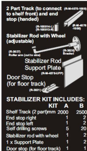
Doors can be made to fit any angle, as the steering of the door is transferred from the usual top track to a track mounted on an interior shelf front.
