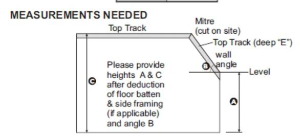
\*The top track is usually fitted to mask the top of the door rather than guide it.
