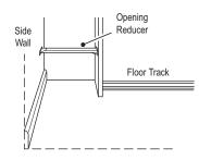
To reduce your opening by more than 457mm / 18" on each side you can construct an 'L' section using an end panel and end fillet. Jointed together with Fixing Blocks and scribed to fit the wall and skirting.
