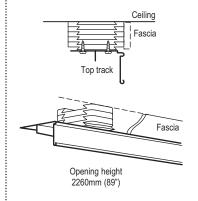
For ceilings between 2399 – 2729mm / 94 ½" – 107 ½" use Opening Reducers. Detailed fixing instructions are provided with each Reducer pack.
