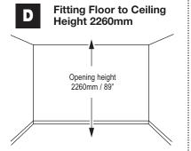
The Top & Bottom Tracksets can be fitted directly to your ceiling and floor using appropriate fixing, which you can buy from any good DIY center.
