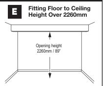
If your ceiling height is between 2272 - 2399mm / 89 ½"- 94 ½" use Spacer Block to reduce it to 2260mm / 89". Detailed instructions are provided with each Spacer Block pack.
