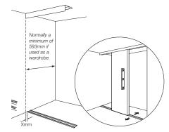
Floor Track - Position the track on the floor of the opening. Mark where holes need to be drilled in the track (we recommend a fixing at each end and centre then at regular intervals in between). Before permanently fitting the floor track to your floor, fit the door into place and using a spirit level adjust the Floor Track so the door becomes
