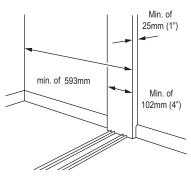
To reduce your opening width by up to 127mm / 5" on each side use Spacer Blocks together with the end fillet and appropriate infill. Detailed instructions are provided with each Spacer Block pack.
