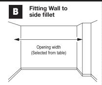
To reduce your opening width from between 127 - 457mm / 5 -18" on each side you can use Opening Reducers fixed to the side wall. Detailed instructions are provided with each Opening Reducer.
