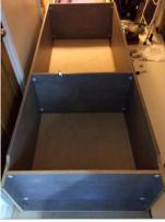
3. The multi drilled holes are at the top of the unit. Three fixed shelves hold the unit together. One at the bottom 5mm holes, a mid shelf first hole of the sequenced multi hole section (4 brackets are provided for additional support on the underside and the very top hole.
