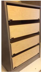
When the box is sitting nice and square push the rod at the front of the runner into the pre drilled hole in the bottom of the box (on both sides).
