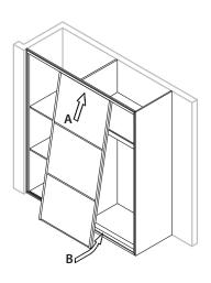
Repeat the process with the front door(s), using the front channel and front bottom track. For multi door systems alternate the doors on the tracks.
